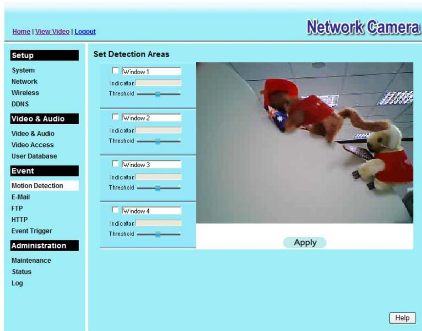
Figure 36: Motion Detection Screen
